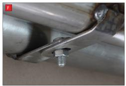
F) When fitting the centre section use the nut and bolt provided to allign the centre pipes and secure them in place.
